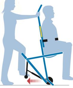
Once at the bottom of the stair, tilt the chair onto the bar and pull the safety wheels out with foot.
