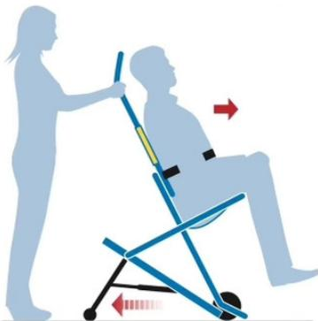
Once chair is secured with four wheels on ground, assist person into chair and fasten safety belts.
