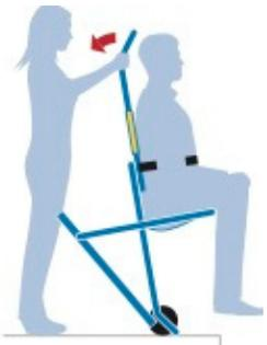
Tilt chair backwards until the wheels engage. Push the chair onto the stairs and lower to match the angle of stairs.
