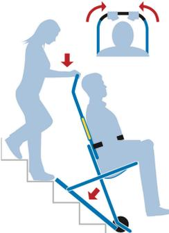
Guide chair down stairs. Weight will be transferred onto the stairs with minimal required effort from person guiding it.
