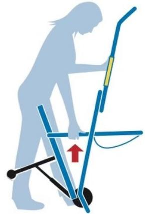
Pull the rear safety wheels into place with foot.
