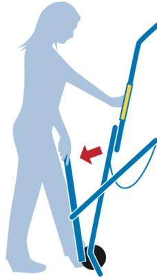
Unbuckle the safety belts, and extend the back leg.
